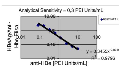
The figures 1a and b show two serial dilutions of the PEI Anti-HBe standard with lot B55C18PT. The calculated analytical sensitivity was 0.30 PEI Units/mL.
